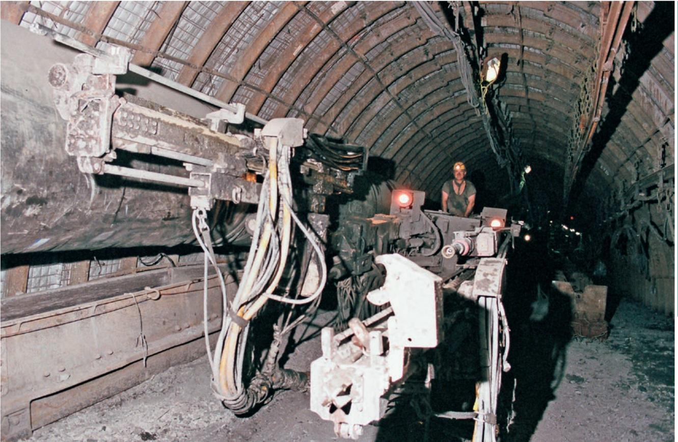
Drilling jumbo BTRK-2 for drilling blasting and block (Hilti) holes
