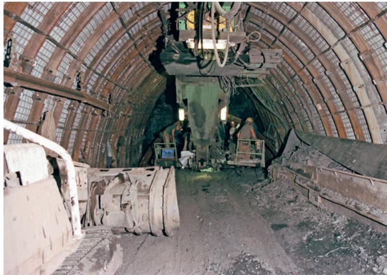
GTA stage AMG 2800, loader K 313 S and crusher with chain conveyor in a drift
