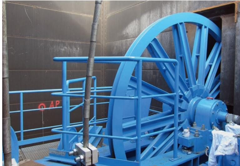
Hoisting sheave platform with rope sheave
