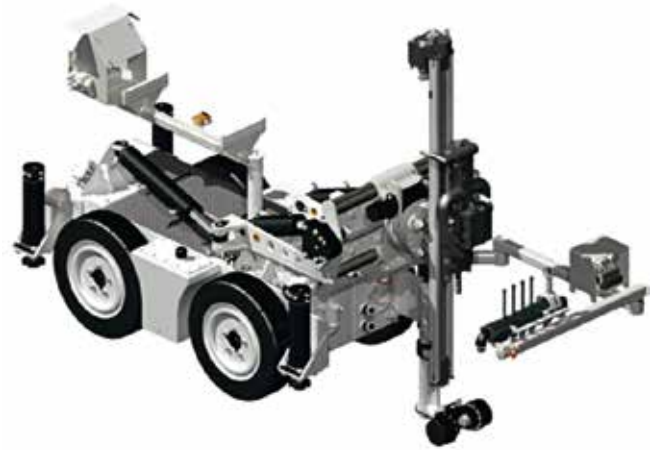
PLH - First pneumatic long hole drill buggy, designed in 1995, now renowned worldwide
