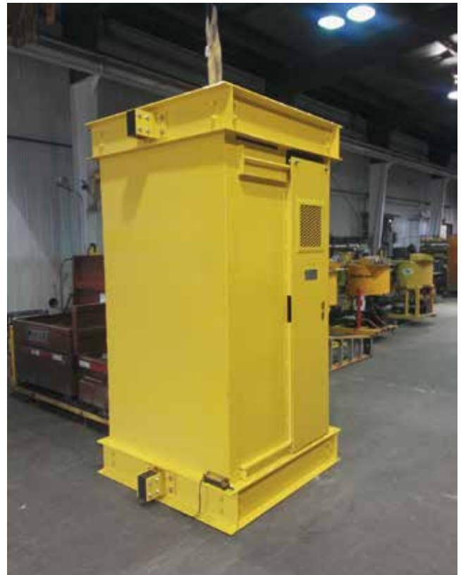
New maintenance cage ready to ship upon completion of plumb test
