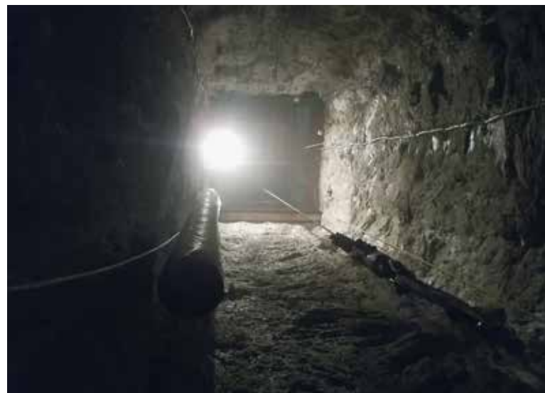
Shaft cross-section and ventilation tube
