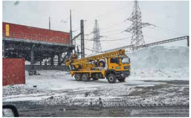
RB50 rotary drilling rig for high-tech deep drilling work
