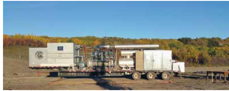
120TR Mobile freeze plant at Mikwan Well Site
