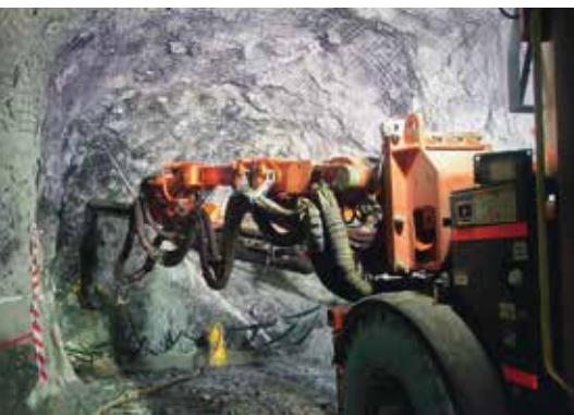
DD422i auto drill in operation
