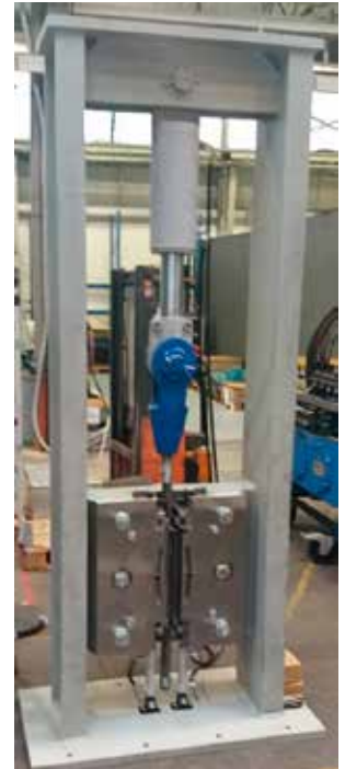
HuK test rig under construction / during assembly
