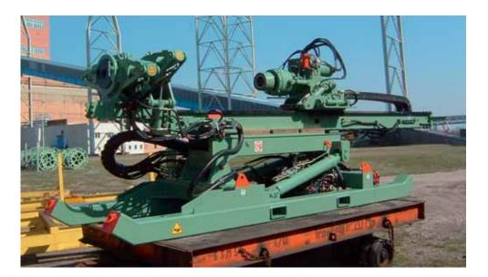
HBR 201 electro-hydraulic drilling machine
