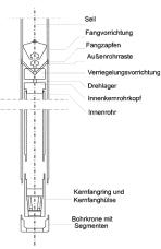
Top: Arrangement of the corebarrel fittings
