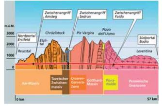
Geological profile along the Gotthard base tunnel
