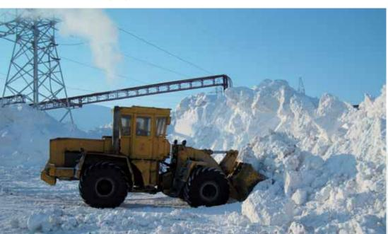
progressed speedily. Some 150,000 m<sup>3</sup> of tundra and loose soil were moved and about 60,000 m<sup>3</sup> of crushed stone ballast laid in place. Preparation work at the shaft site was therefore practically completed by the autumn of 2008. A tipping point was also set up to accommodate the sinking debris.
