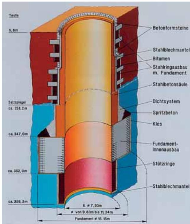
Top: Schematic diagram of the inner support system in the freeze zone
