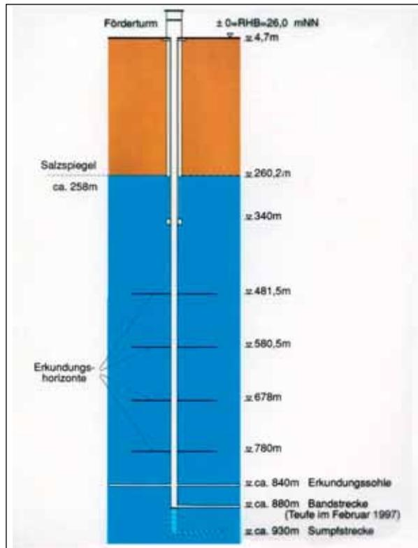
Right: Schematic diagram of shaft no. 1
