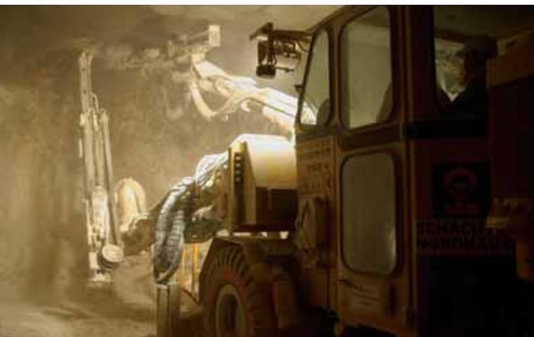
Drilling blasting holes and bolt-setting holes
