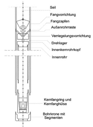
Top: Arrangement of the core-barrel fittings
