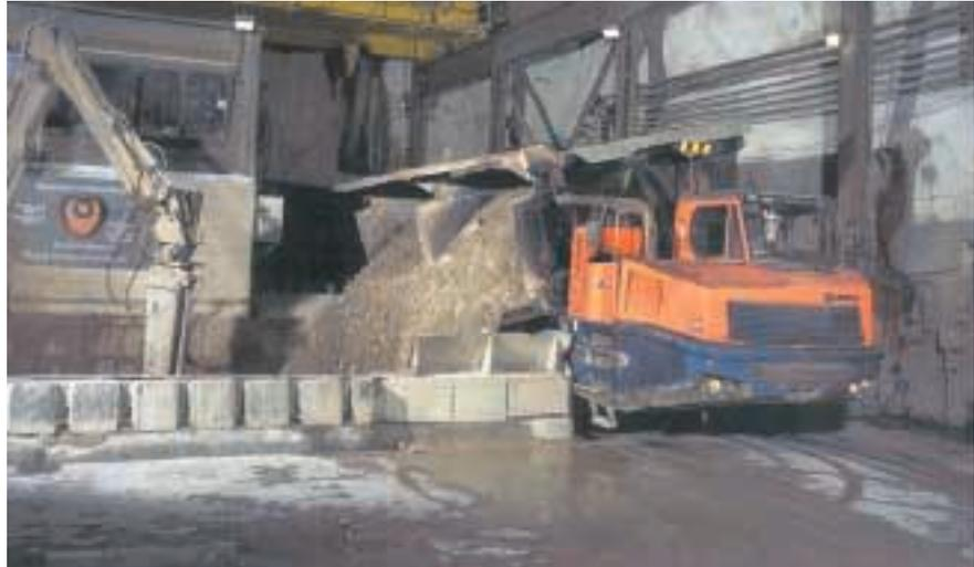
An 80 ton side-dumping Tamrock Supra truck tipping its load into the underground crusher in a matter of seconds
