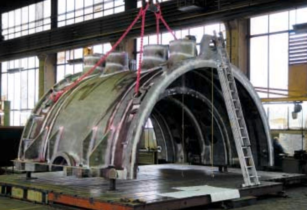
to build another low-pressure housing with a surface area of 13.9 m<sup>2</sup> and a component weight of about 80 t.
