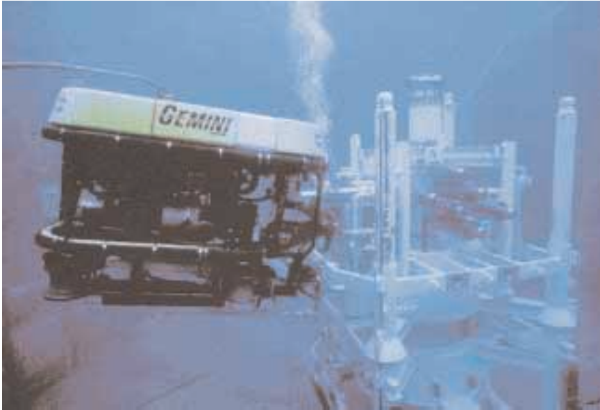
Rov positioning a Christmas Tree on the sea bed
