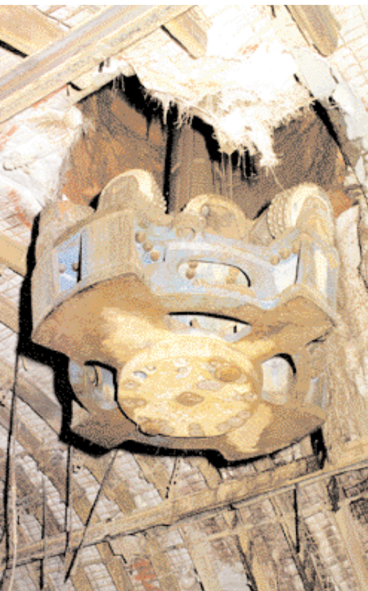
Raise boring, 1.8 m ø raisebore head, level 20
