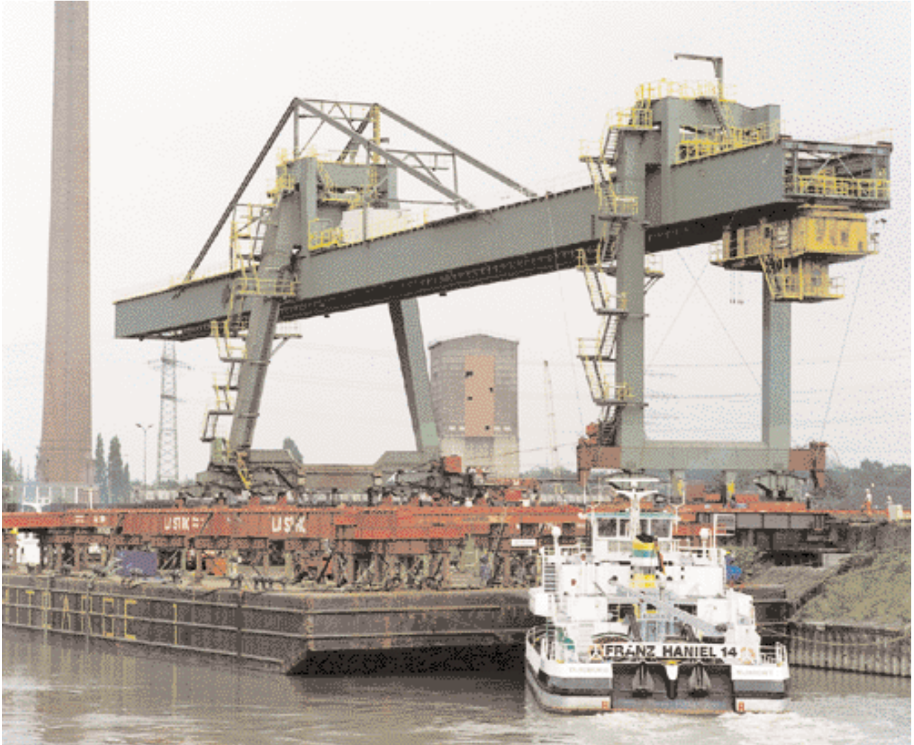
Travelling crane is "shipped out"
