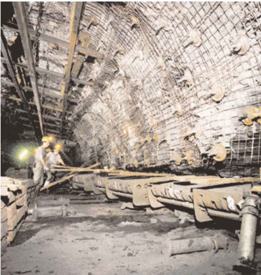
Picture above: Ready-assembled shield-support columns wait in the main seam road
