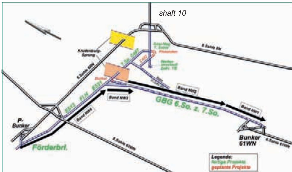
Pic. left: Volumetric picture Prosper-Haniel mine, area Shaft 10: western elements of the tunneling concept
