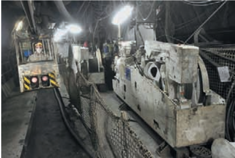
Sinking winches and diesel trolley operations
